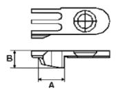
Short finger for 5.2 mm not available Short finger for 6.0 mm 236101A46009 Thick finger for 5,2 mm 236101C45209 Thick finger for 6,0 mm 236101C46009
